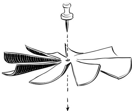
3. Using a push pin, attach the turbine to a straw at one end (illustration at right). Leave space (or insert washer, if needed) between the straw and the turbine, so it spins freely.
