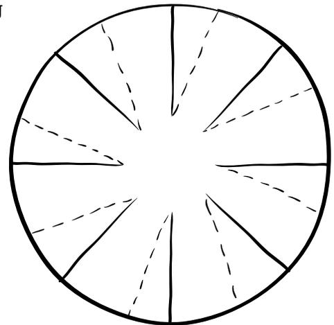
2. Taking each blade, bend one side gently up (along the dashed lines) so that all blades are curved up the same direction. (Pick a direction, such as clockwise, and stick to it all the way around). Don't overwork the blades at this point. You may need to make adjustments to the bend of the blades when you start using your turbine.
